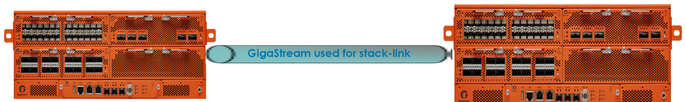
Figure 4 Daisy-Chain Configuration using GigaStream for Stack-link
